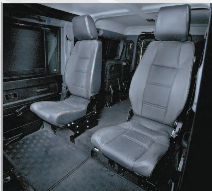
Two outside seats with walk-through isle shown providing easy access to rear lock and fold seats.
